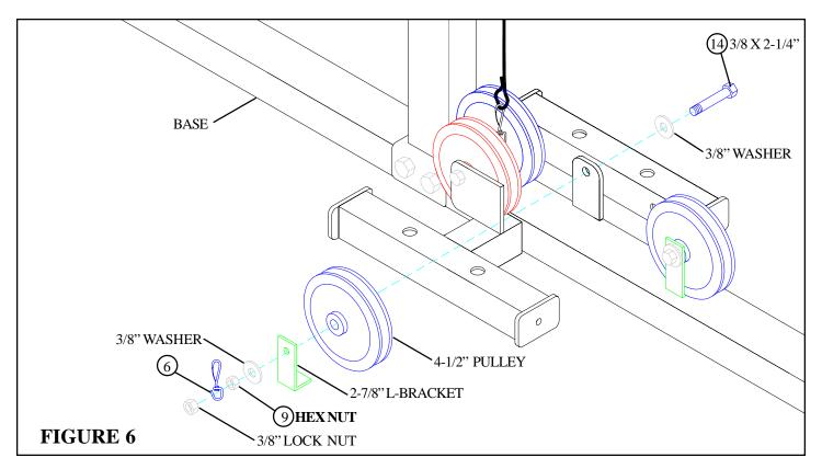
• **SECURELY** assemble the previously removed 4-1/2" PULLEY to the BASE using one 3/8 X 2-1/4" BOLT (14), two previously removed 3/8" WASHERS, one previously removed 2-7/8" L-BRACKET, one SWIVEL SNAP (6), one 3/8" HEX NUT (9), and one previously removed 3/8" LOCK NUT. See FIGURE 6.
